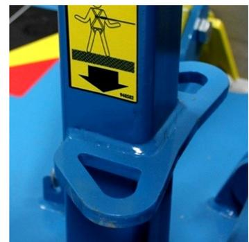
Travel restraint anchoring rings
