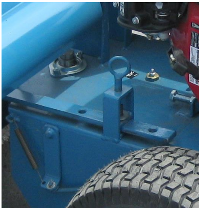
Fig. 3 Brush direction control
