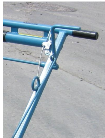
Fig. 6 Wheel and brush engagement lever
