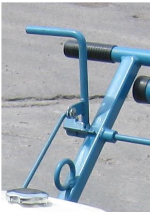
Fig. 5 Wheel engagement lever
