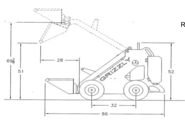
Weight: 1190 lbs With bucket: 1310 lbs Tipping capacity: 1000 lbs Rated operating capacity: 500 lbs (50% of tipping capacity)
