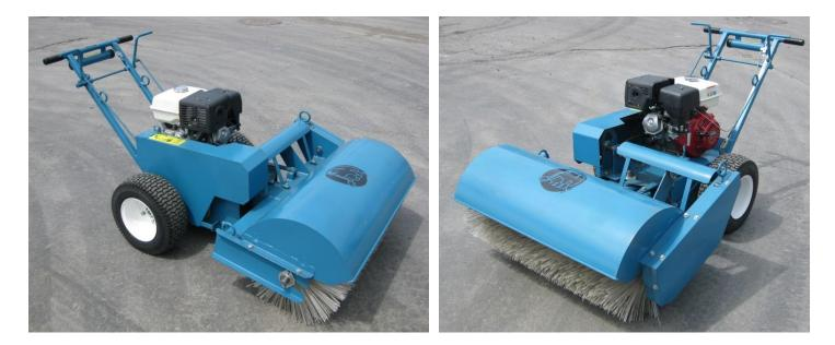
Independent and adjustable engagement of wheels and brush Differential with 1'' axles 16 sealed ball bearings throughout 16 X 6.50-8 wheels #50 chain driven brush with self adjusting chain tensioner 4 lifting rings Reinforced brush cover
