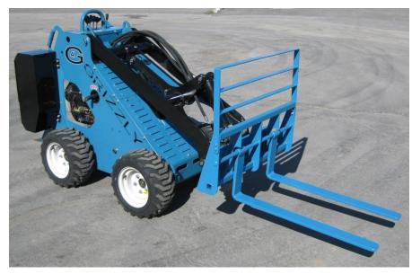
An interesting addition to your G41.. An efficient way to transfer skids of light material, rolls, bundles or whatever can be loaded onto or picked up by these forks.
