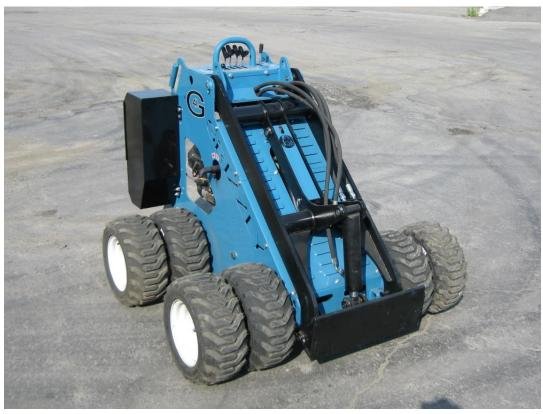
This dual wheel kit is EASY ON, EASY OFF! This simple option allows the weight of this already light machine to be spread over eight wheels allowing it to work over soft or fragile surfaces with more confidence. Operator is ultimately responsible for working on any surface and must proceed with care.
