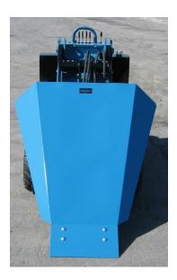
This roof remover attachment will lift the old material over its back plate to allow the material to be picked up at a more comfortable height, to be discarded into trailer or workhorse.
