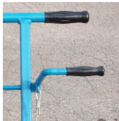
Fig. 6 Wheel and brush engagement lever
