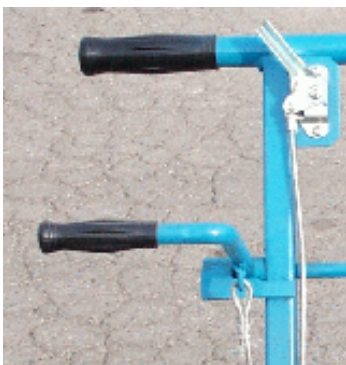
Fig. 5 Wheel engagement lever
