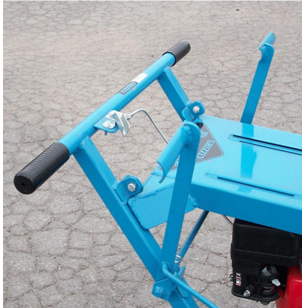
Fig. 3 Levers in brake on, clutch disengaged position
